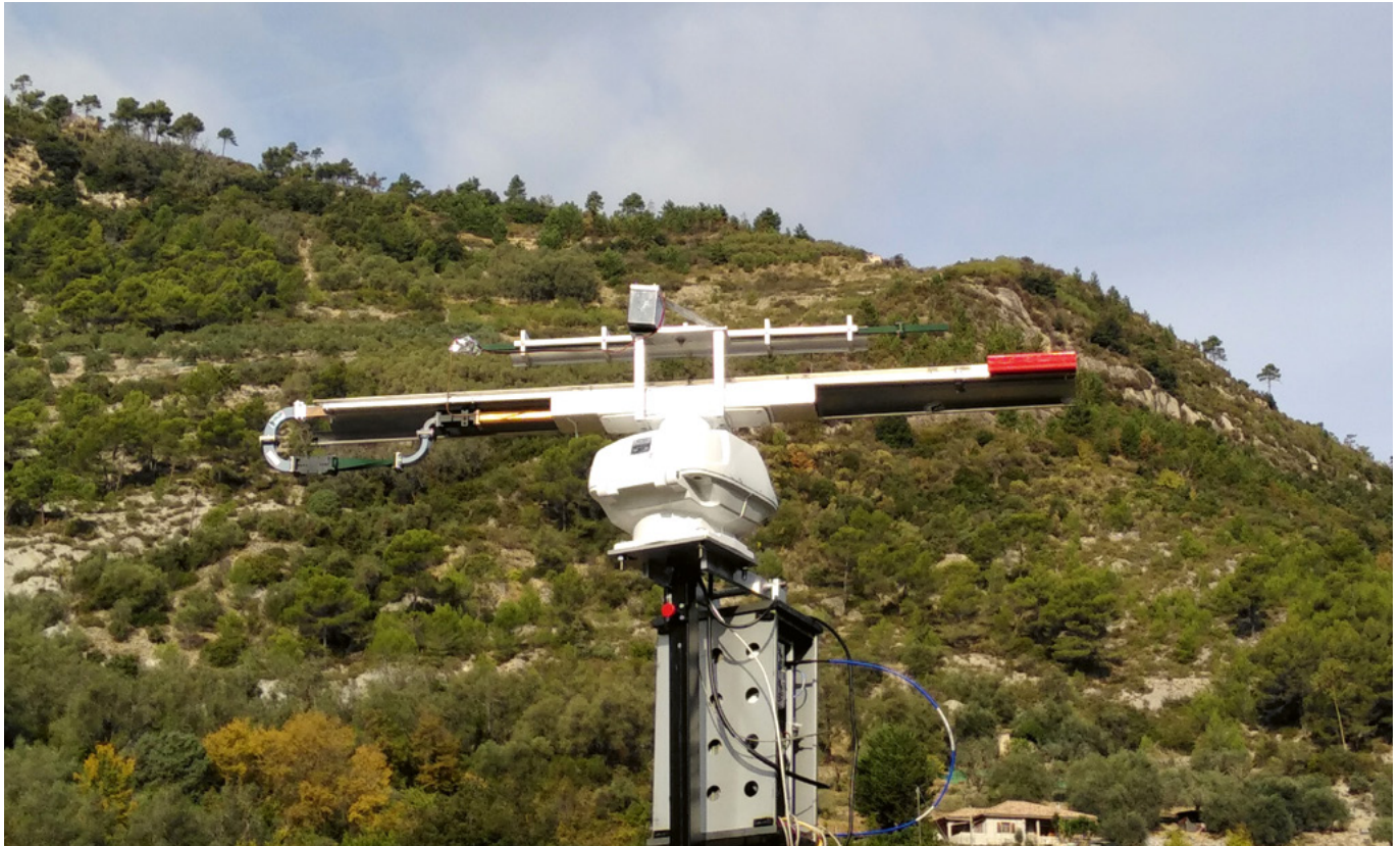
Figure 8: The harmonic radar developed within the STOPVESPA project [©LIFE STOPVESPA].
